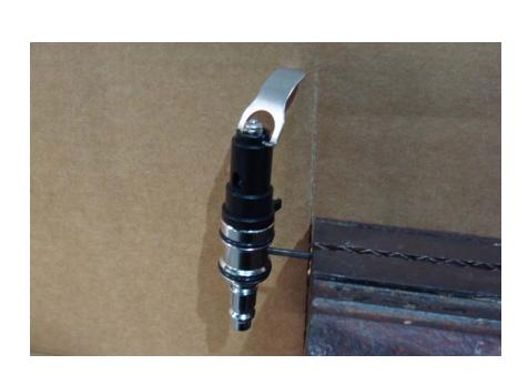
After removing the regulator valve body from the Gemini housing, you will need to secure it in a vise.
