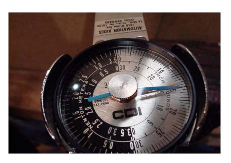
Using an inch-pound torque wrench, torque unit to 15 inchpounds. This will provide the proper amount of torque to prevent the two housings from unthreading, which causes the leak.
